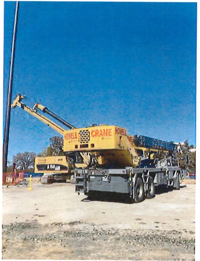
Truck mount crane to place reinforcement for pier Ed Carrigan Dec 11, 2024 12:16 PM
