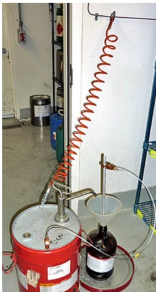
This image shows dispensing into a glass container. Note the ground rod inserted into the funnel.
